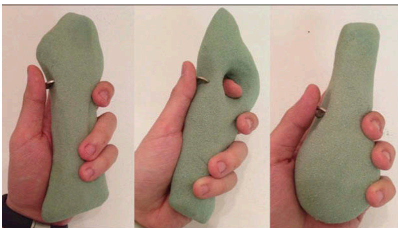
Figure 1. This figure depicts the foam models and the small marker for thumb control placement used in the design and construction of the cane handle.
