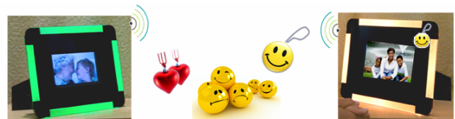
Figure 2: Aurama is an interactive photo frame emitting colored light auras and uses intelligent photo frame jewelry that provides explicit awareness of affections, status, emotions
