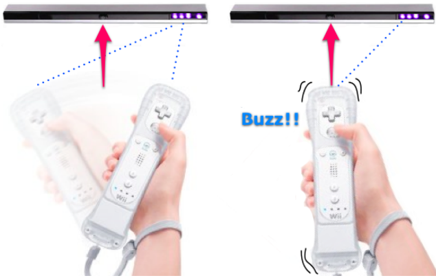
Figure 4: Tactile dowsing: the player moves the Wii remote in the horizontal plane (left); The closer the Wii remote points to the target direction the more continuous the perception of vibrotactile feedback will feel (right).
