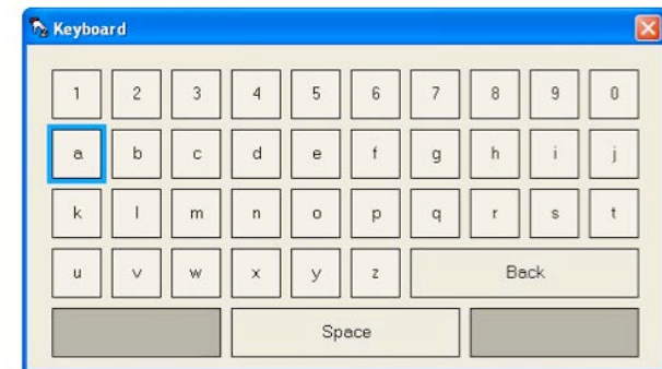
Figure 6. The selection keyboard used in our experiment. This keyboard was based on 3 selection keyboards from Microsoft's Xbox. Here the selector is positioned over the letter "a." The dark buttons are Xbox-specific and were not used in the study.
