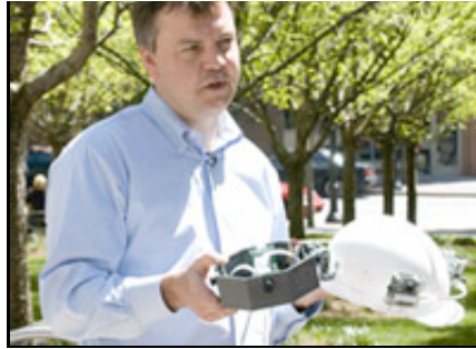
Frank Dellaert shows prototypes of SWAN's computer vision system. The white hard hat with the cameras is an early proof of concept prototype of the computer vision system. The gray octagonal box is the next iteration of the computer vision system.
