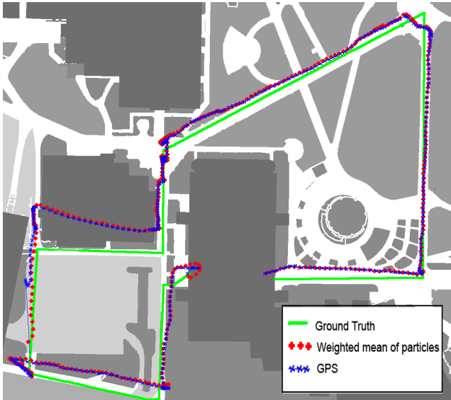
Fig. 1. Tracking without using a map prior on the first dataset. Note that the particle trace is almost coincident with the GPS trace.
