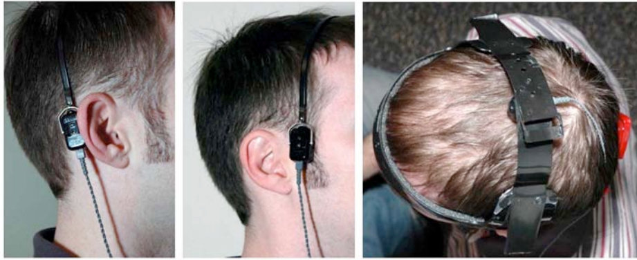
Figure 4. Headband bracket for securing the RadioEar B-71 BC transducer (shown), for use in mastoid (left image), condyle (center), and vertex (right) locations.
