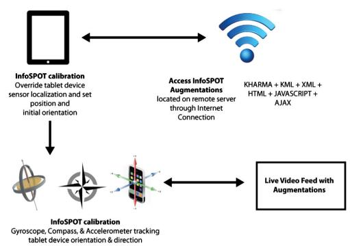
Fig. 8. The InfoSPOT system architecture.
