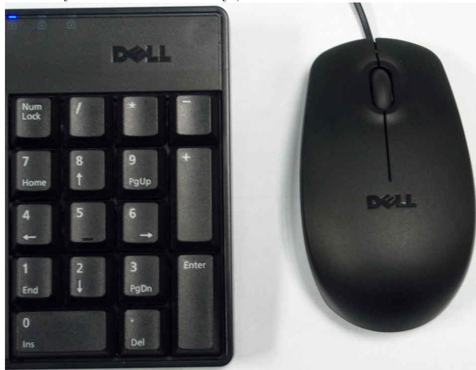
Figure 15: The mouse and the right side of the keyboard used in the experiment. Note the additional keys around the number keys, and the horizontal tactile mark on the 5 key.
