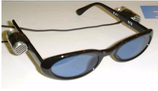
Figure 7. Pre-amplified microphones for capturing real world sounds
