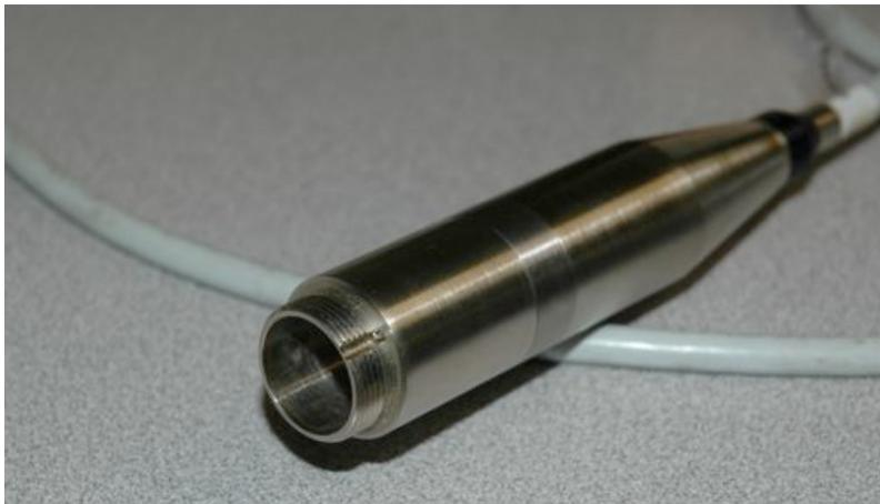
Figure A1. *2cc coupler, microphone (B&K Type 4146), and connector housing used in this study. These separate components are visually separated by different shades of metal. They are attached via matched threads.*
