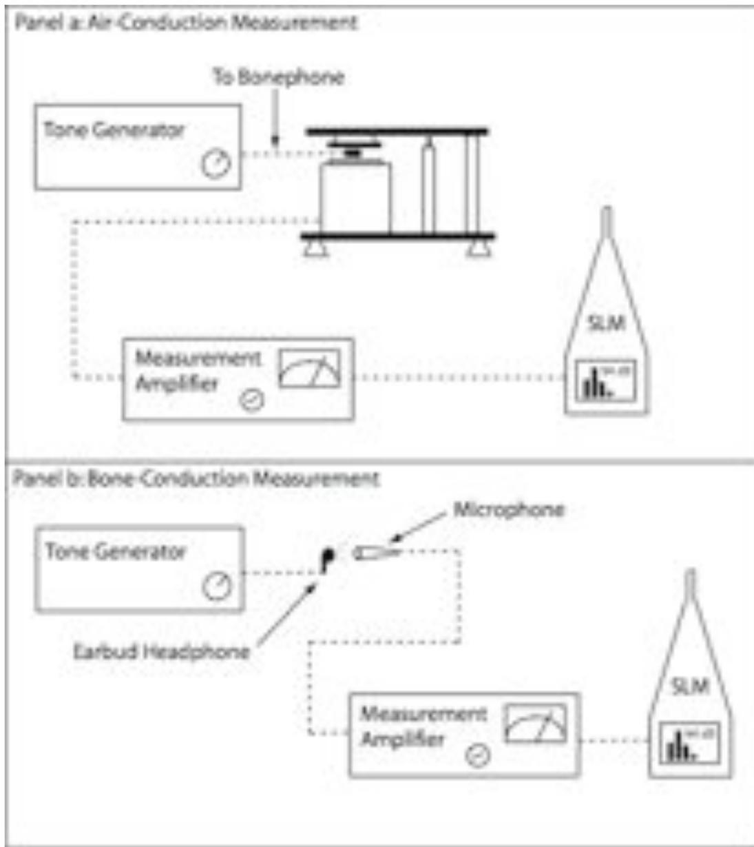
Figure A7. Measurement setups for air and bone conduction.
