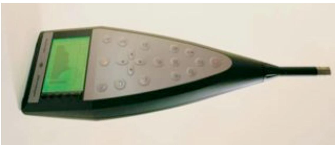
Figure A3: *Sound level meter used in this study: Brüel & Kjaer Type 2260.*
