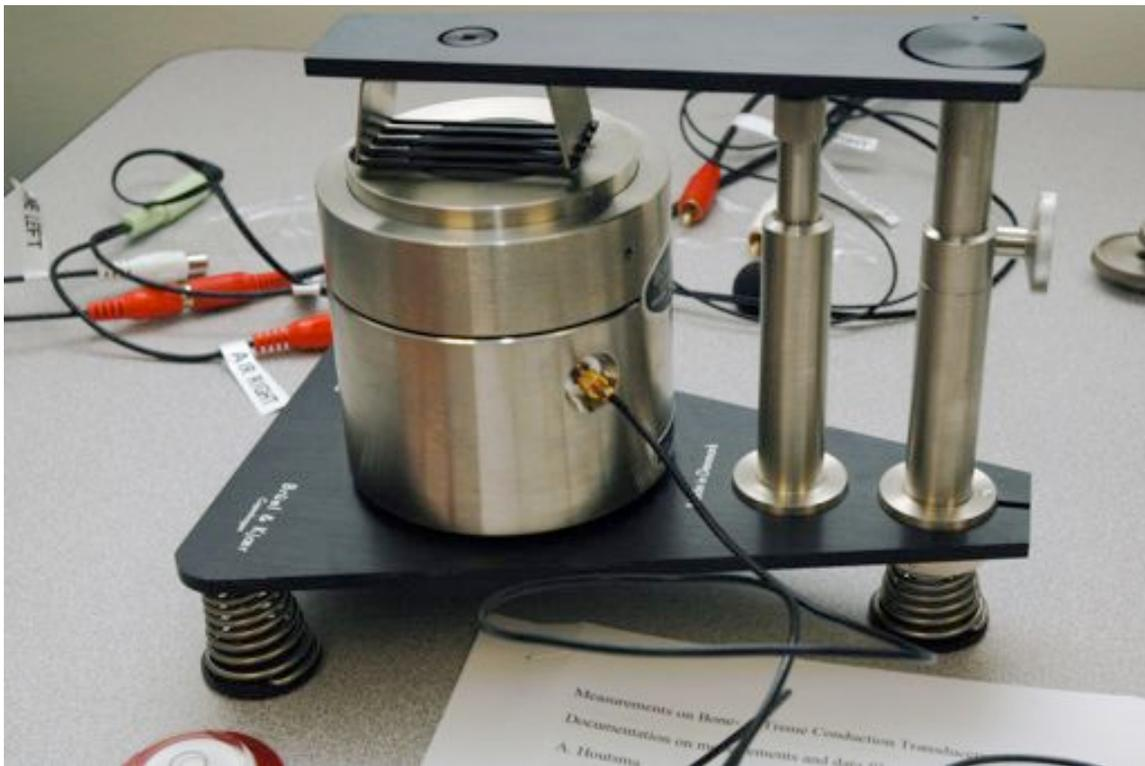
Figure A4. *Artificial mastoid used in this study: Brüel & Kjær Type 4930.*
