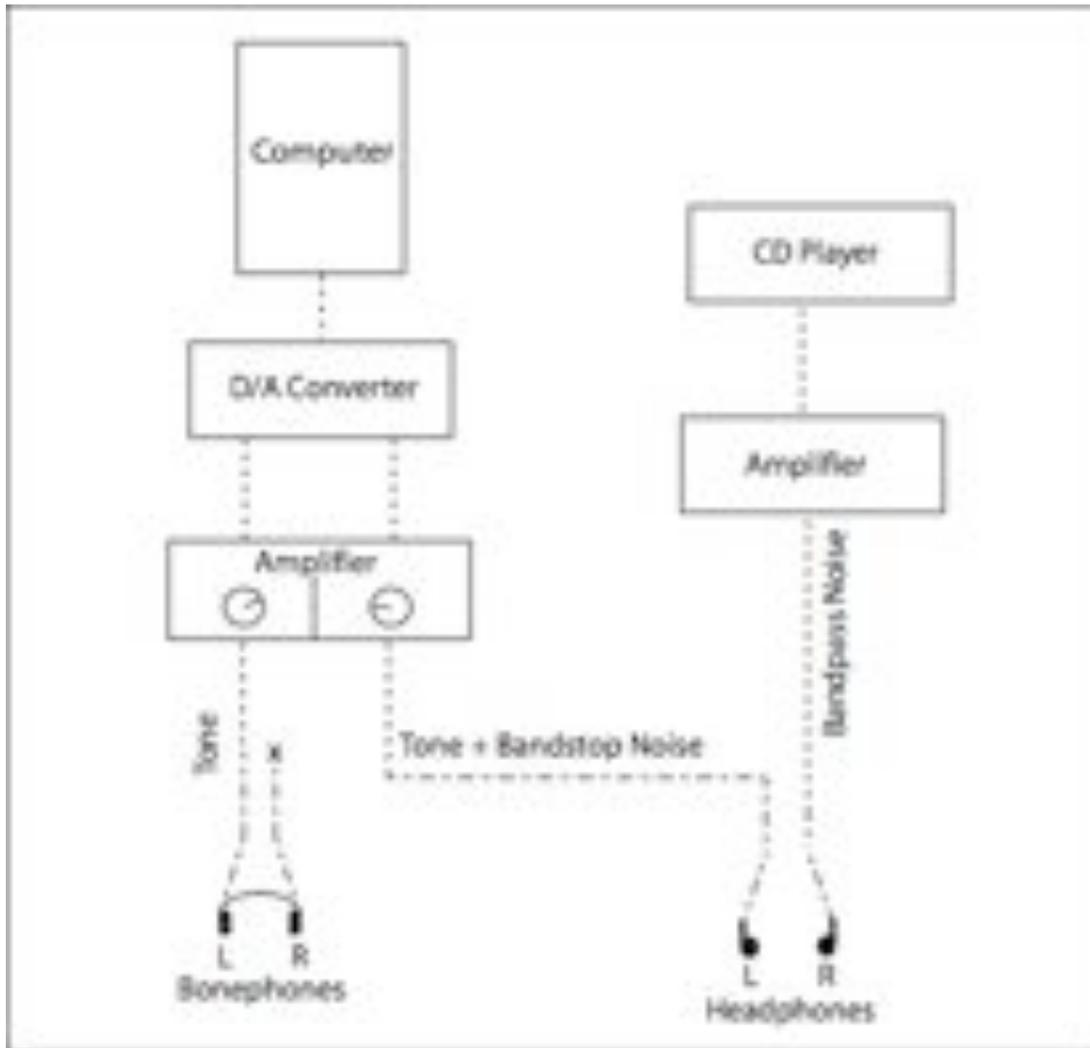
*Figure 6.* Sound delivery apparatus in this study. In this schematic, the left ear is the test ear, and the right ear in the non-test ear. The tones and bandstop noise originate from the computer and get sent to the left ear (the test ear) of the appropriate transducers. The bandpass noise originates from a CD player and is sent to the headphone on the right ear (the non-test ear).
