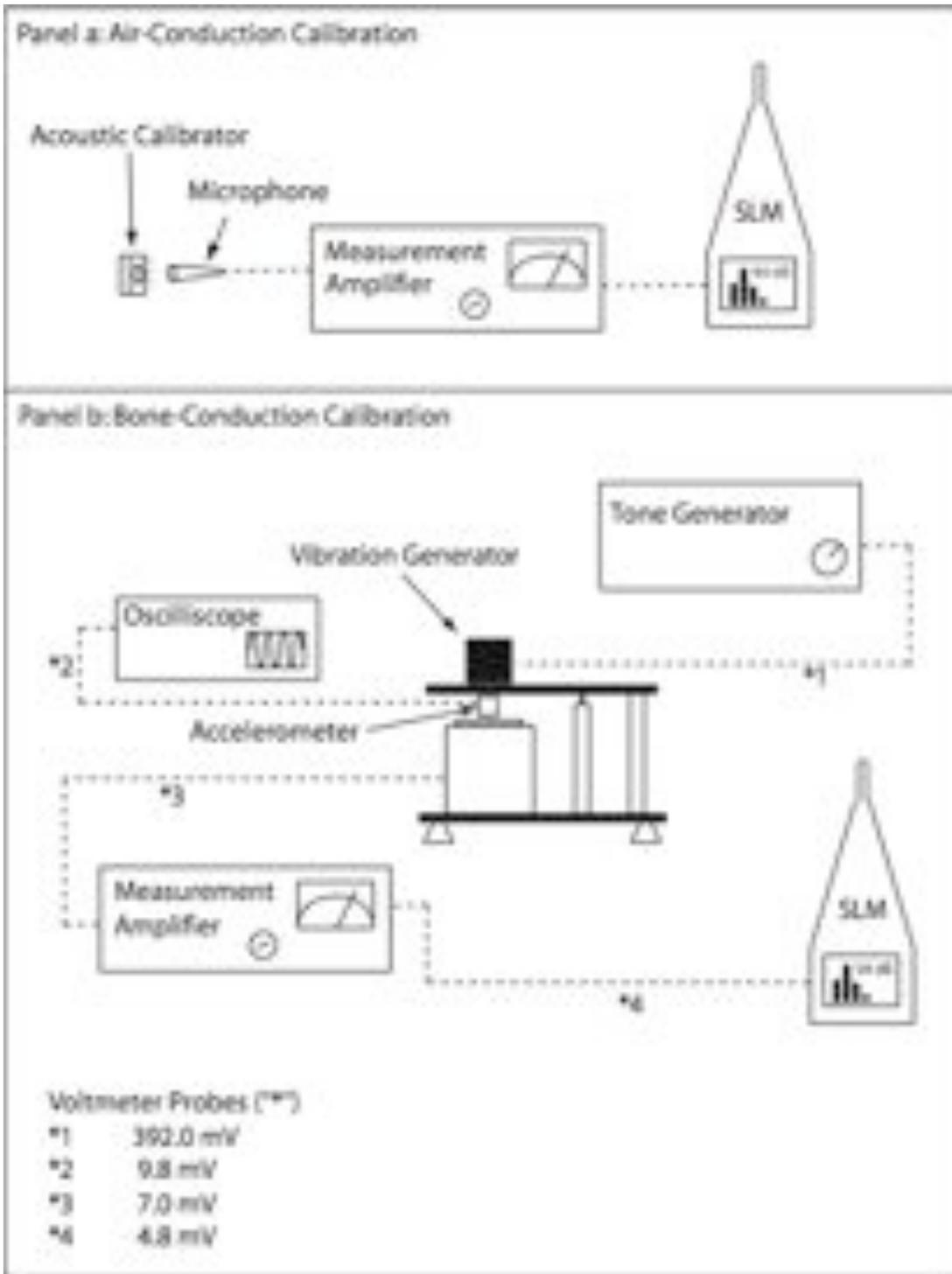
Figure A6. Calibration setups for bone conduction and air conduction. “\*” followed by number indicate voltage probes into system.
