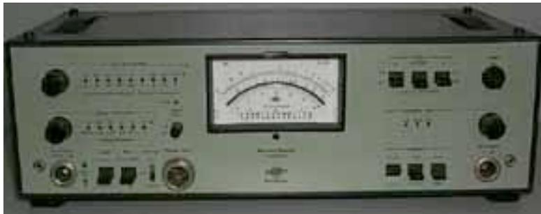
Figure A2. *Measurement Amplifier used in this study, Brüel & Kjaer Type 2610.*
