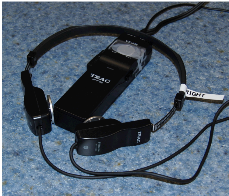
Figure 2. Photograph of Teac HP-F100 “Filltune” bone-conduction transducers used in the present studies.
