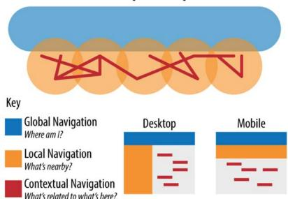
Building context—allowing users to locate their positions within the system—is a critical function of navigation systems.
